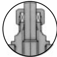
Stuffing box construction for sizes 3/8 to 1
